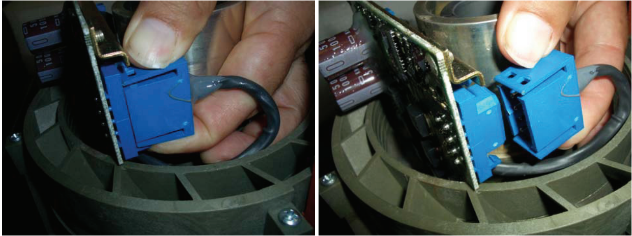
Figure 5.6-21 Detail, Removal of Printed Circuit Board Connector
